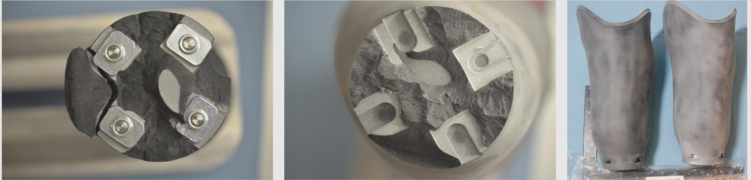
Printed with HP's MJF technology and HP's 3D HR PA 12 material
