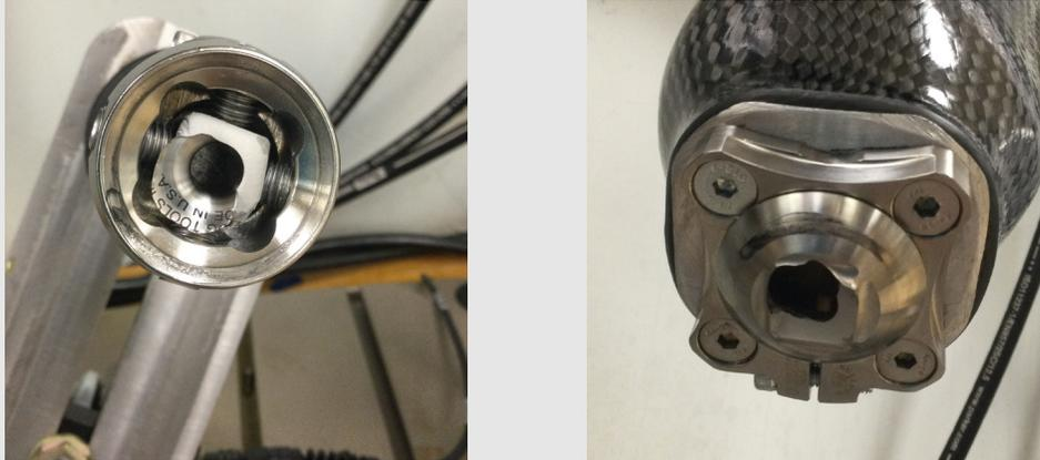
Fig. 6 These images show how and where the titanium pyramidal adapter failed
