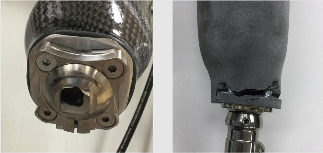
Images above are the failures endured after a cyclic fatigue test, as defined in the below chart. Image on the left shows the carbon fiber socket and image on the right shows socket printed using HP's MJF technology and HP's 3D HR PA 12 material.
