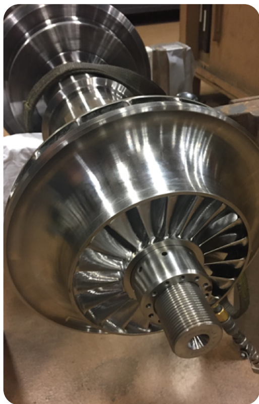
The Hanwha shrouded impeller assembled on a rotor shaft
