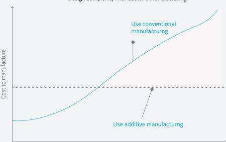
With conventional manufacturing, as the degree of complexity increases, the cost to manufacture also increases. Additive manufacturing eliminates this factor, so design innovation is essentially free.
