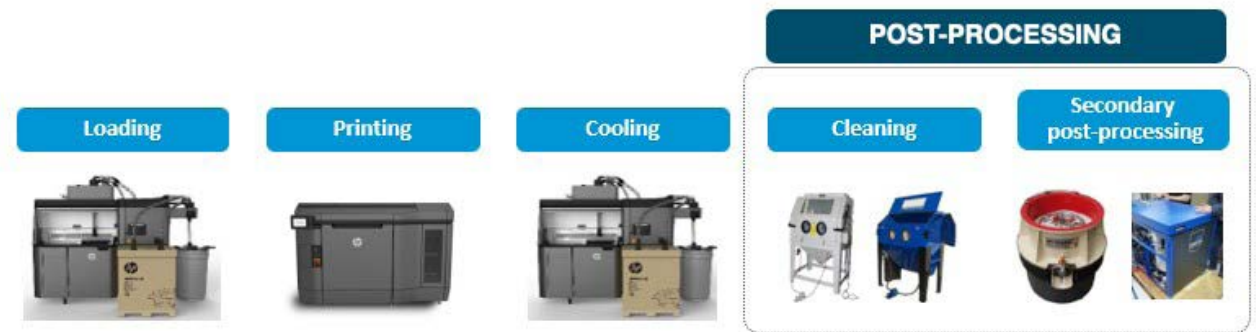
Figure 1. E2E HP Jet Fusion 3D Printing workflow
