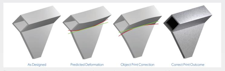
The simulation engine analyzes the design, predicts deformation in the print, and applies a counter-deformation to the part, so the part comes out right the first time and every time. It also predicts part risks and failures, validating the execution feasibility of the print prior to starting the build process.
