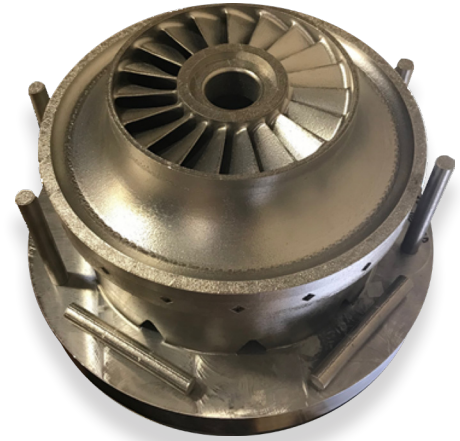
The turbine wheel still attached to the build plate as it came out of the Sapphire metal AM printer.
