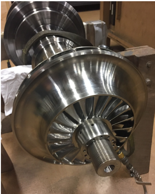
The Hanwha shrouded impeller assembled on a rotor shaft
