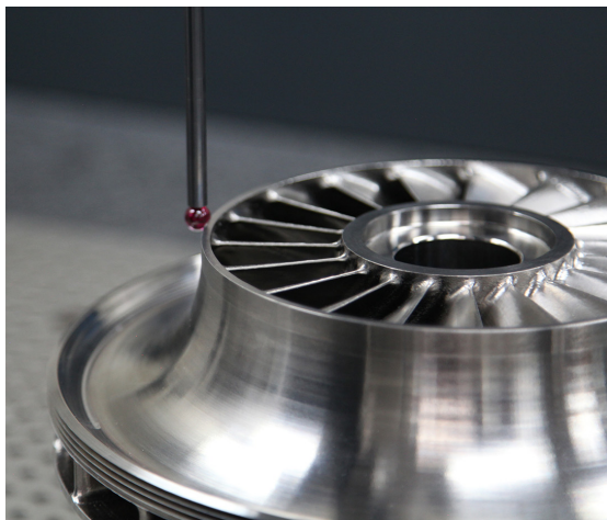
Stratasys Direct ensured accurate dimensional measuring of the shrouded impeller with a Coordinate Measuring Machine (CMM)
